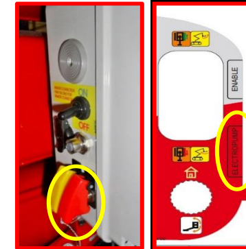
Picture 29: electropump activation buttons.
