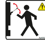
Picture 70: indication of emergency manual pump.
